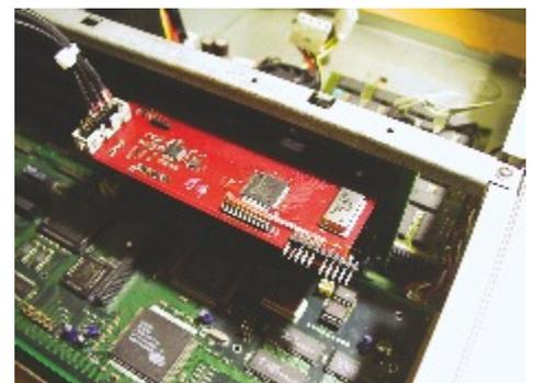
*Prisma Megamix installed in A4000*
